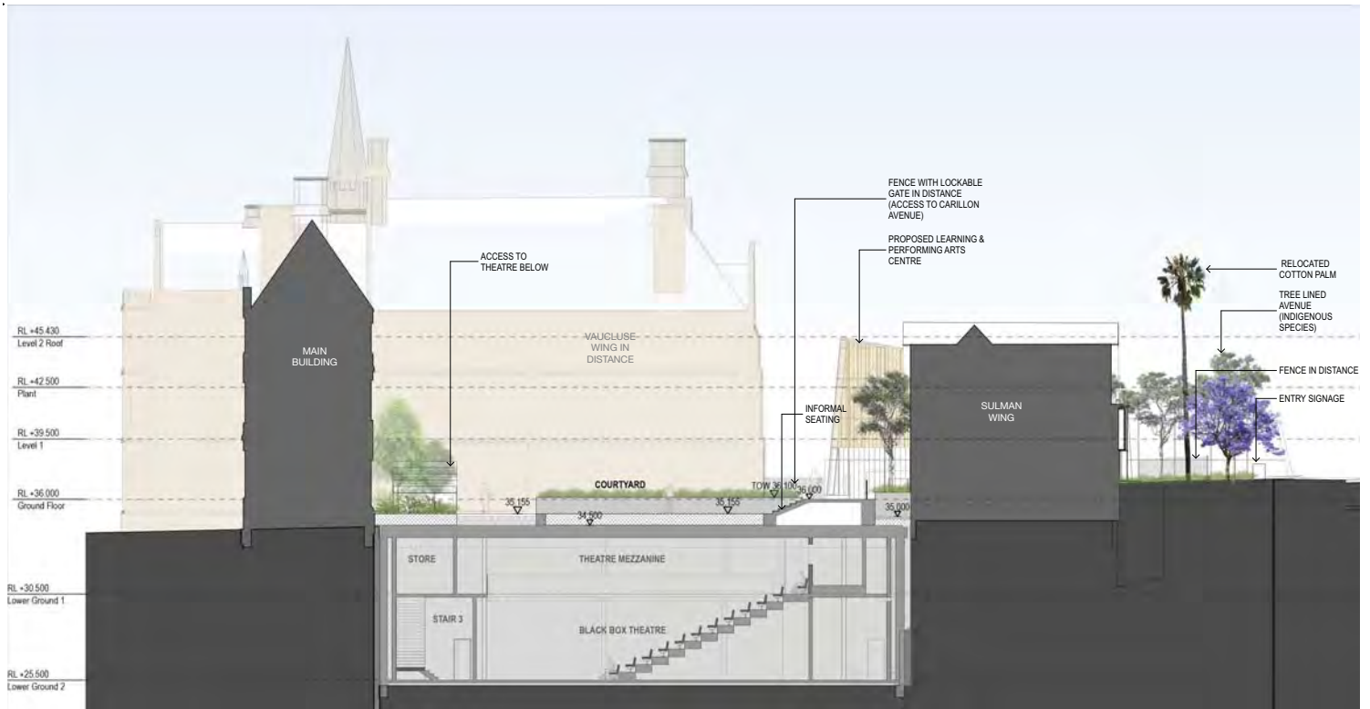
A SECTION / ELEVATION Section A 1:200
